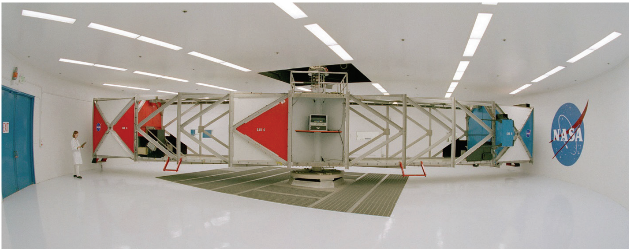
The 20 G centrifuge at the NASA Ames Research Center
